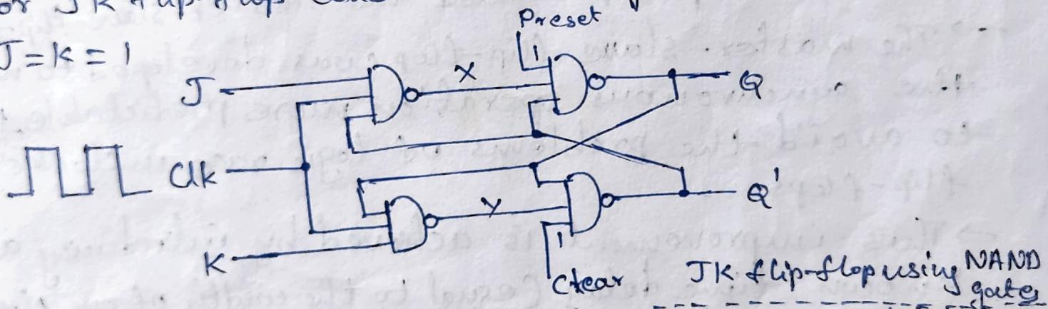
→ If the width of the clock pulse  $t_p$  is too long, the state of the flip-flop will keep on changing from 0 to 1, 1 to 0, 0 to 1 and so on, and at the end of the clock pulse, its state will be uncertain. This phenomenon is called race around condition.
