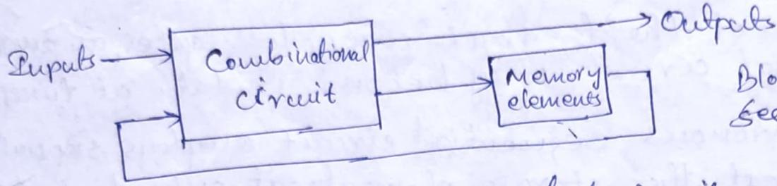
Block diagram of Sequential Circuit
