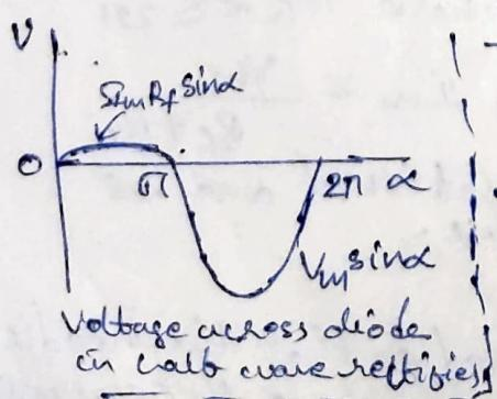
→ When diode is conducting, it has a resistance  $R_f$ , and voltage across it is  $iR_f$
