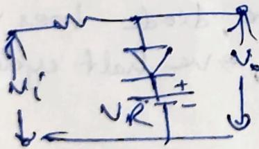
b) Biased positive clipper with reverse polarity of battery \$V\_R\$
