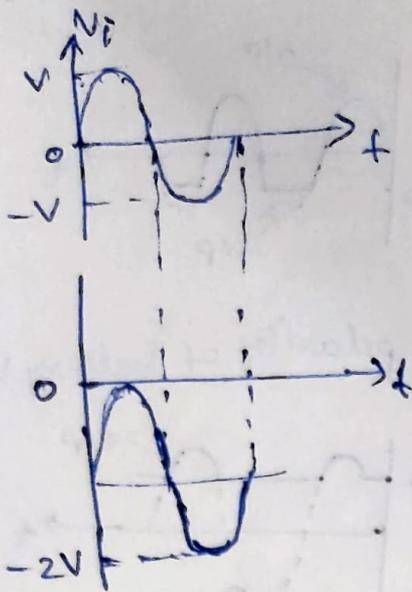
→ During +ve half cycle, the diode conducts, i.e. it acts like a short ckt.
