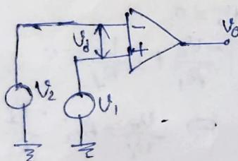
→ Since the gain is infinite, the off voltage  $V_o$  is either at its positive saturation voltage ( $+V_{sat}$ ) for  $V_1 > V_2$  or negative saturation voltage ( $-V_{sat}$ ) for  $V_2 > V_1$ .
