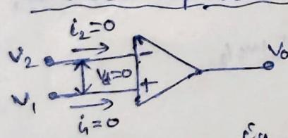
→ If  $V_1 = 0$ , o/p  $V_0$  is  $180^{\circ}$  out of phase with i/p signal  $V_2$
