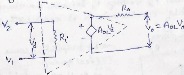
→ So the equivalent circuit of an op-amp may be shown as above, where  $A_{OL} \neq \infty$ ,  $R_i \neq \infty$ , and  $R_o \neq 0$
